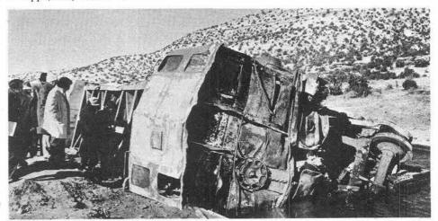
September. The cask and car were then moved and reassembled at the same tilt angle in a concrete-lined pool where burning JP-4 jet fuel floating on water engulfed the cask in flames that produced heats of 1800 to 2100°F. The railcar eventually warped in the intense heat and turned over into the pool, but the cask survived a 90-minute fire period during which it was exposed to six times the heat input required by current qualification test standards.
